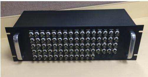
Overcomes the 15 volt bias on ICP Accelerometers and allows multiple recorders to be directly connected.
