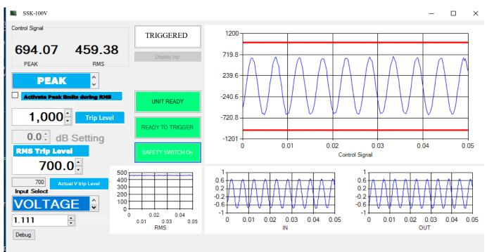
The system displays real time the monitored signal and both the supply signal coming in and going out of the unit. No more uncertainty if the signal is present.
